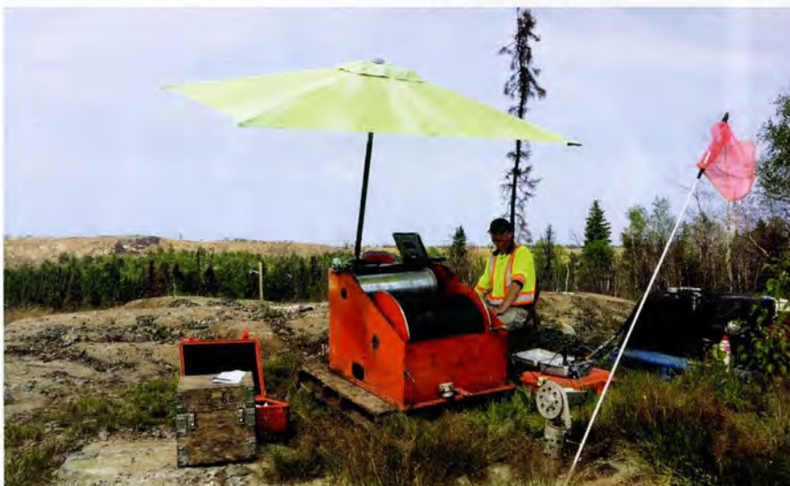
Rob Chapman staying cool while conducting a borehole survey.
