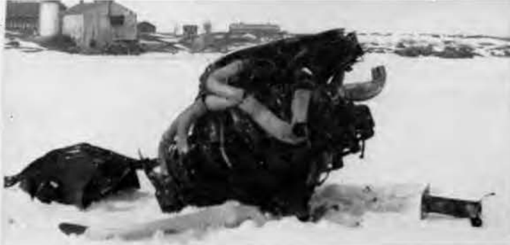
Lac du Bonnet, Good Friday, 1936. Motor tore away from fuselage and made parabola over and behind burning aircraft.
