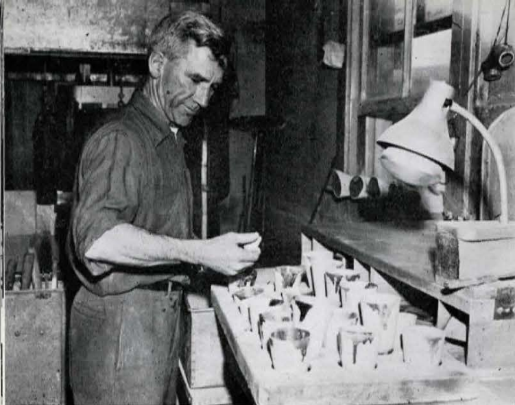
Jim Foley adds reagents to crucible before firing.
