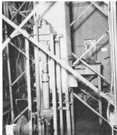
Fluo-Solid Roaster (lower portion) Feeder.
