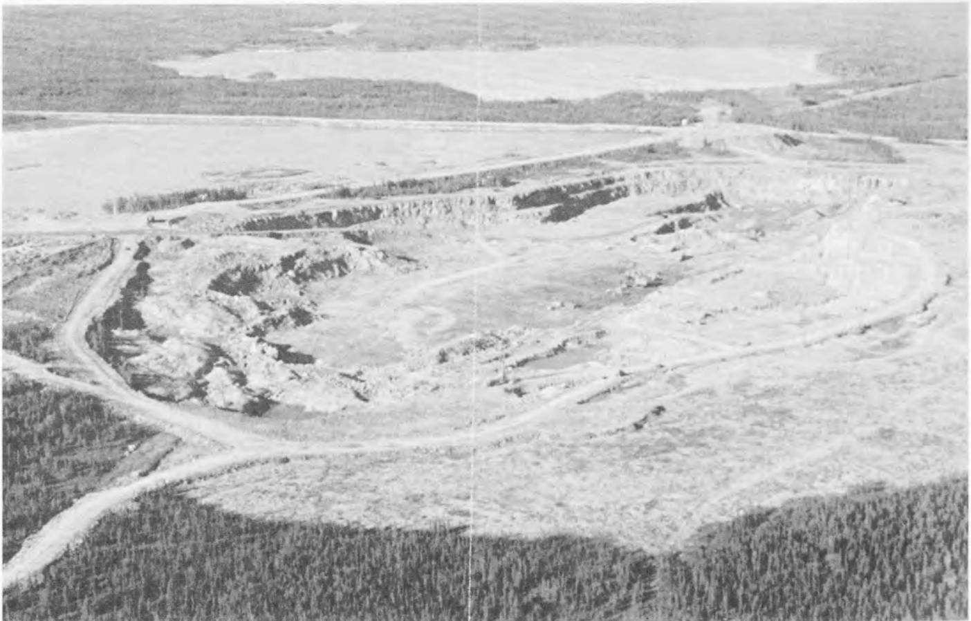
The open pit at Ruttan Mine where 50,000 tons of ore and waste rock must be removed every day.
