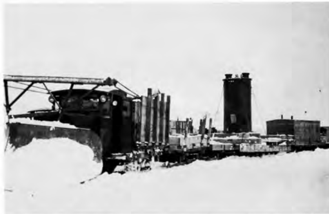
Linn tractors were equipped with snow plows and were capable of hauling up to 38 tons, the weight of this load. The huge transformer had to be transported on a specially built rack. (F. Willis 1928)
