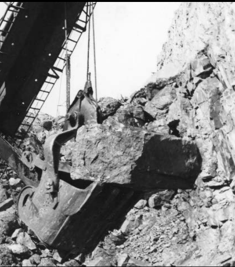
The Marion electric shovel (shown here hard at work in the open ore pit) was used in a variety of different locations of the mine. 1930s.
